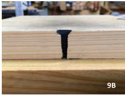
Figure 9 – A side view of a properly countersunk pilot hole (a) and with black paint added (b) to highlight the resulting pattern.
