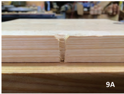
Figure 9 – A side view of a properly countersunk pilot hole (a) and with black paint added (b) to highlight the resulting pattern.
