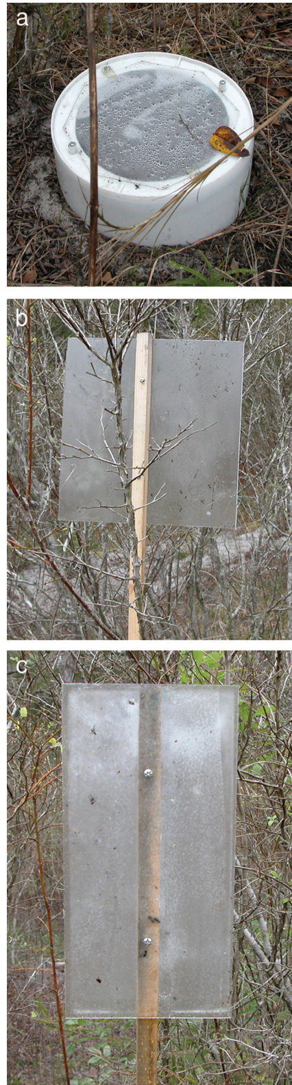
Fig. 1. Trap types: (a) bucket emergence trap, (b) panel trap, and (c) modified panel trap. (Online figure in color.)
