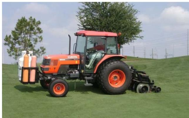
**Figure 16.** Equipment used for applying Curfew Soil Fumigant to turf.
